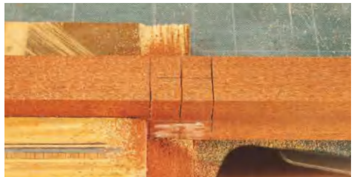
▲ Pic.12 Sawing the third stick down to the chalked squares
